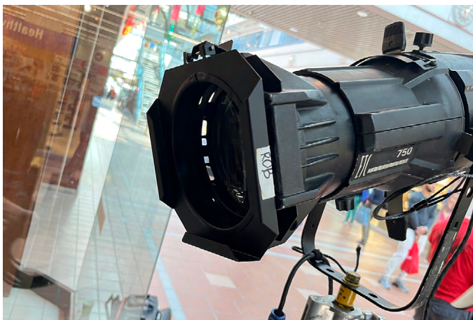
1253 Adapter attached to a Source 4 fixture on set.
