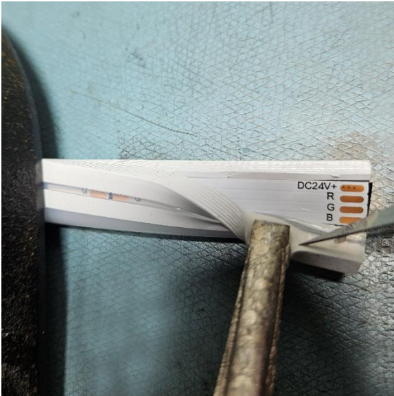
Figure 10: Use your exacto knife to cut away a portion of the interior plastic window strip carefully
