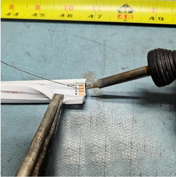
Figure 13: Using your soldering iron, lightly “tin” the pads
