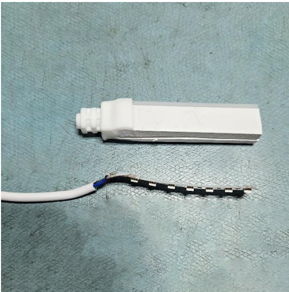
Figure 4: The original tails can be used by carefully removing and reattaching them
