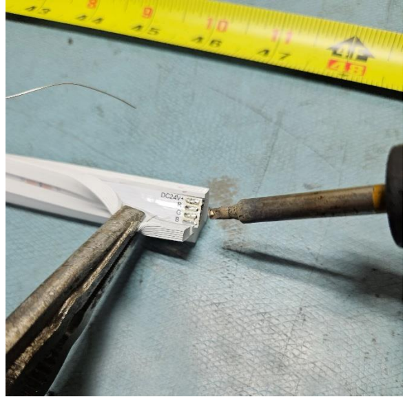
Figure 14: Coat the pads with a small amount of solder
