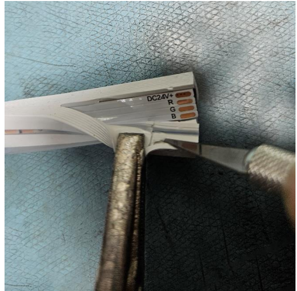
Figure 11: Slice through the plastic, then carefully slide the blade behind the plastic to free it from the silicone
