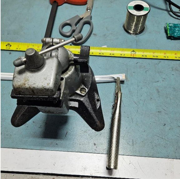
Figure 8: Use a clamp or vice grip onto one edge of the silicone
