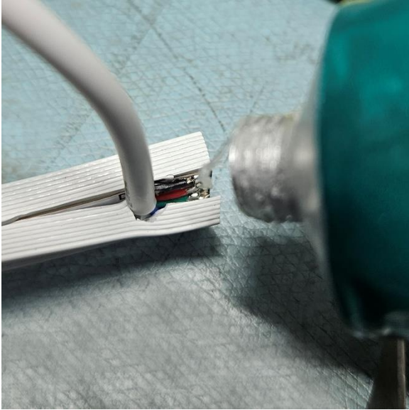
Figure 20: Use silicone to fill in the cut as well as possible
