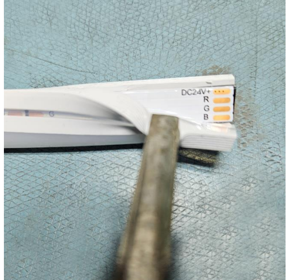
Figure 9: Make sure the copper pads are easily accessible
