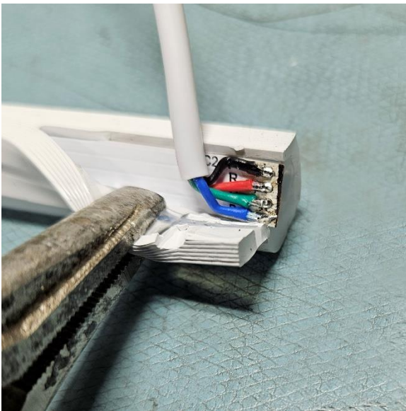
Figure 17: Carefully bend the main body of the wire to your desired angle
